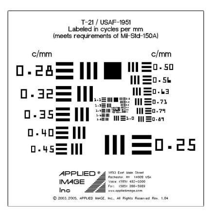
The T-21 has labels which state the actual cy/mm of each element, so no look-up table is needed.
