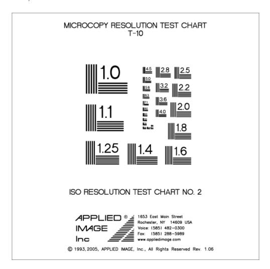
The T-10 is marked directly in cy/mm and is used extensively in the microfilm field.
