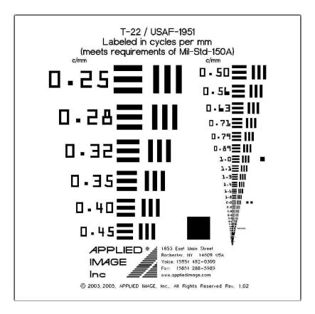
The T-22 further improves the pattern by arranging the elements in straight lines (much easier to locate, much easier to scan). Of course, it still meets the requirements of Mil-Std-150A. Finder squares have been added to help determine which element is being viewed, when the labels cannot be clearly seen.
